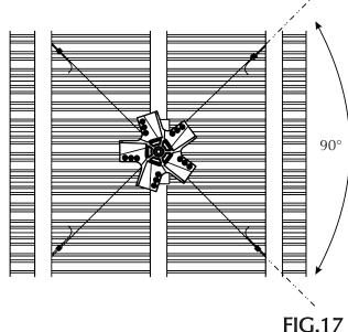
NOTE: Fans hanging lower than 10 ft from where the guy wires will mount will require additional cable.
